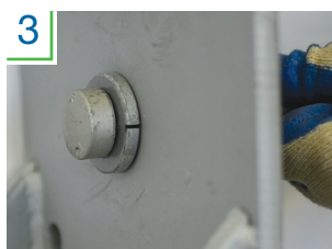
3 Pulling back, rock the tool side-to-side to engage the collapsible washer.
