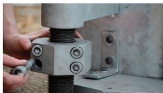
Insert all four socket screws to join halves and hand tighten
